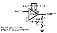
NOTE:  $R_1 || R_2$  indicates the parallel combination of  $R_1$  and  $R_2$ .
