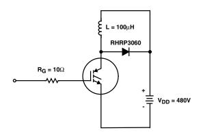
FIGURE 16. INDUCTIVE SWITCHING TEST CIRCUIT
