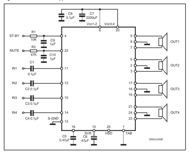
Figure 1: Standard Test and Application Circuit
