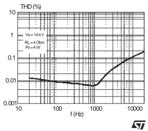
Figure 9. Distortion vs. frequency.
